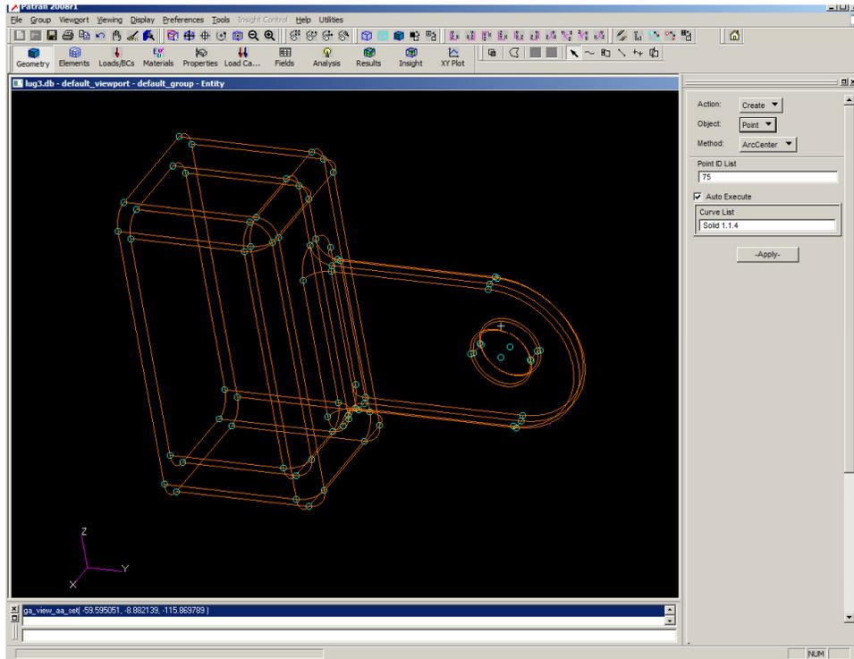
The first coordinate system is created by *Geometry, Create, Coord, 3Point* using origin, point on Axis 3 and point on Plane 1-3 as shown:
