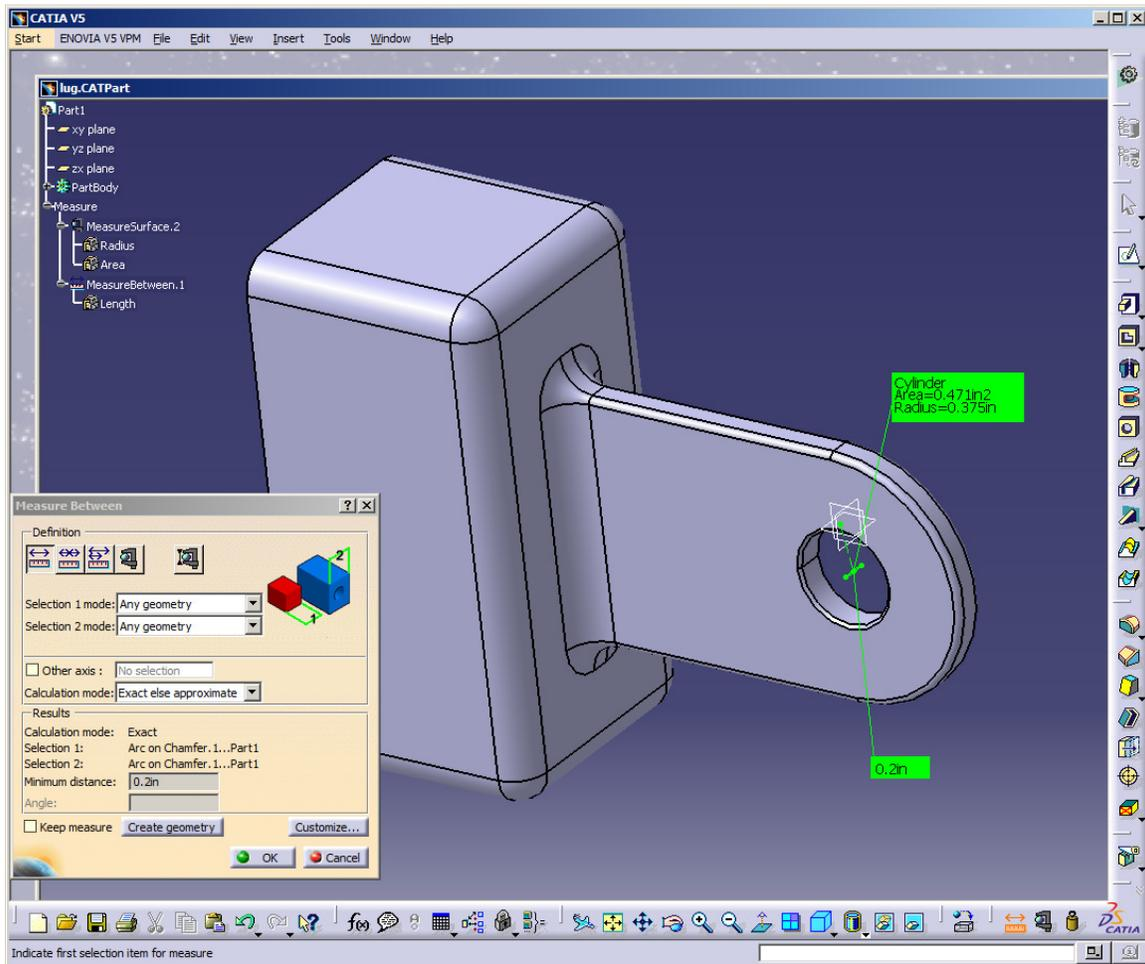
Although the lug is 0.25in thick, chamfers reduces the bearing surface to 0.2in. The above geometry was created in CATIA, and imported into PATRAN:
