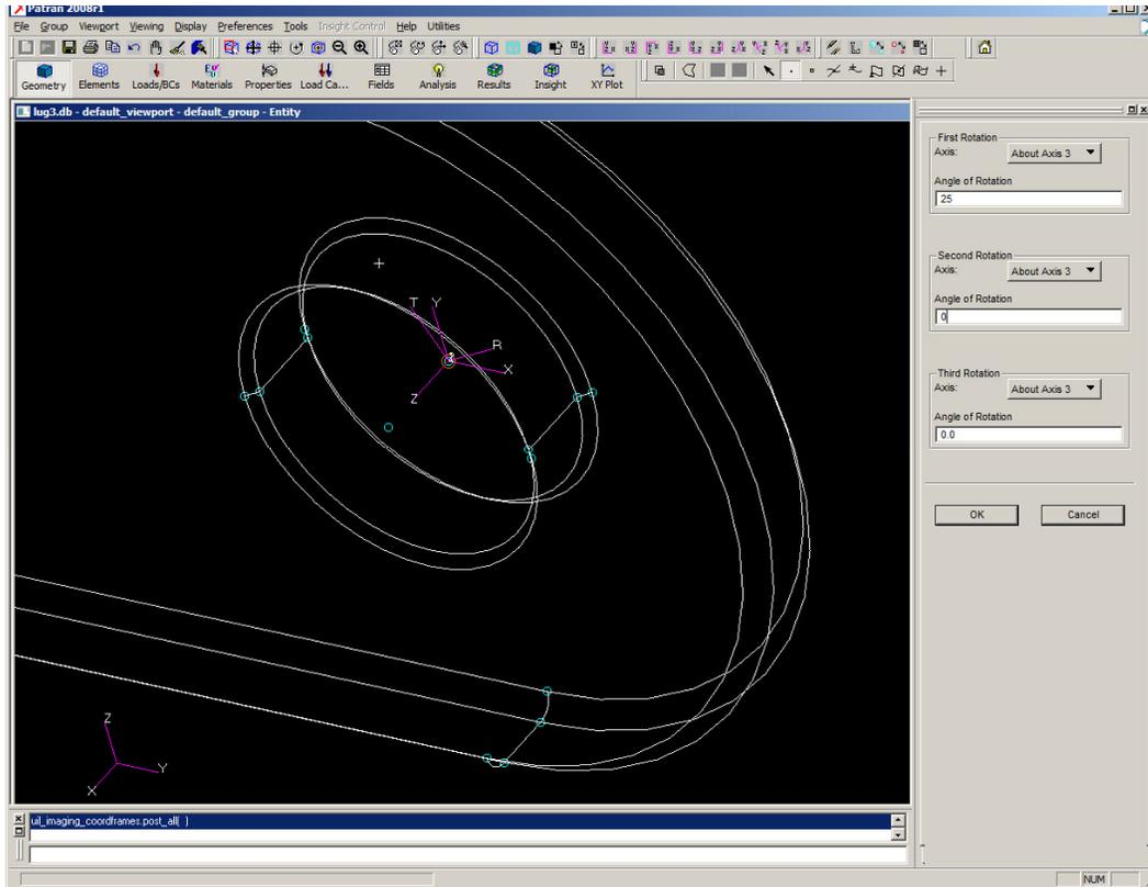
With the desired coordinate system created, a field can now be defined. A pressure load can be created to apply normal pressure to selected surfaces (in this case the cylindrical surfaces) with the magnitude controlled by the field.
