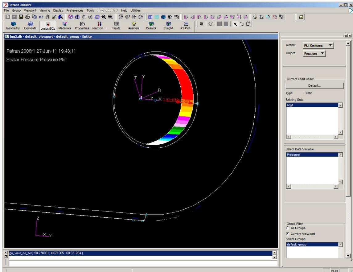
For expedience, we may simply ground the end (*Loads/BC, Create, Displacement*) and submit the model to the NASTRAN solver:
