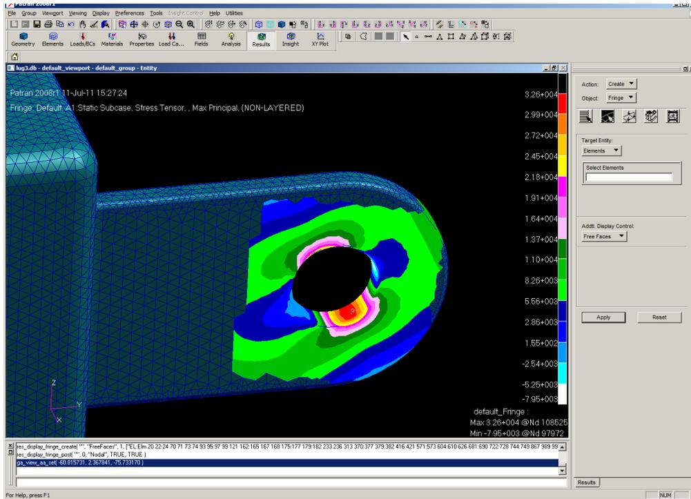
By comparison, the non-linear solution presents a maximum stress at the radius of 47.0ksi:
