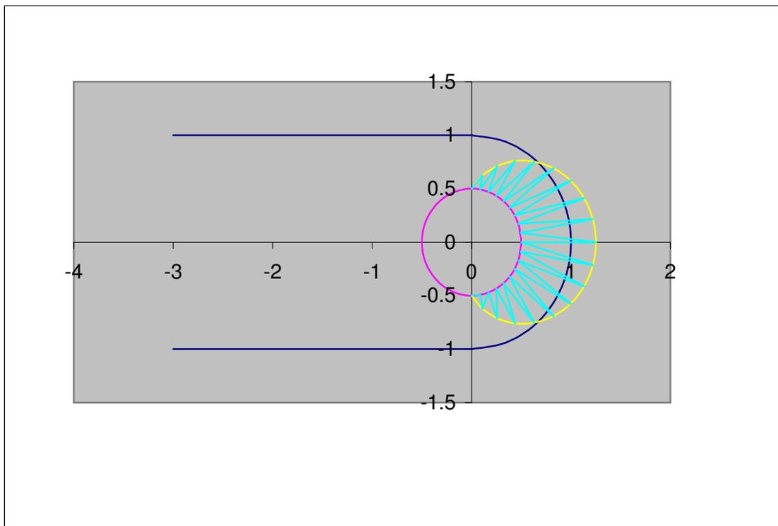
A common simple approach is to assume that the surface pressure on the 180 degrees portion of the hole in compression follows the equation:
