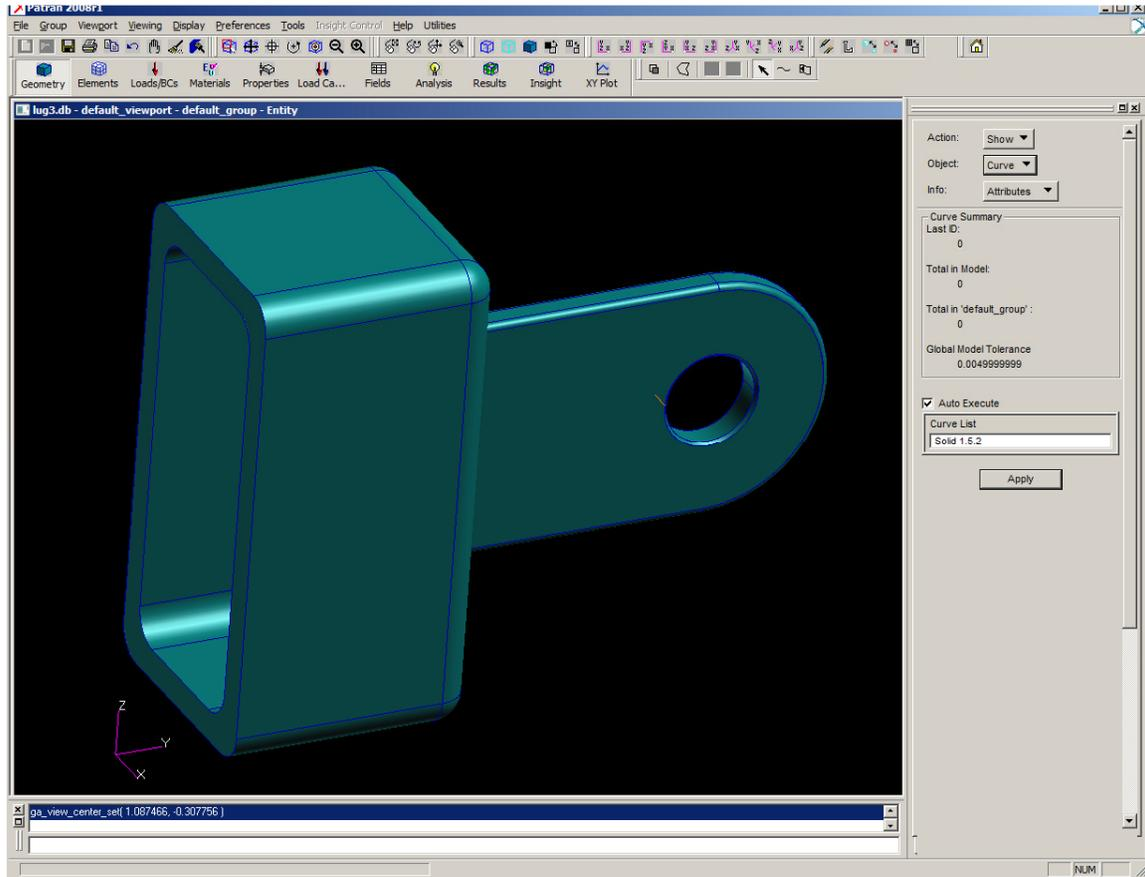
To apply the load, first a rectangular coordinate system is created at the center of the hole. Next, a cylindrical coordinate system is created rotated 25 degrees.
