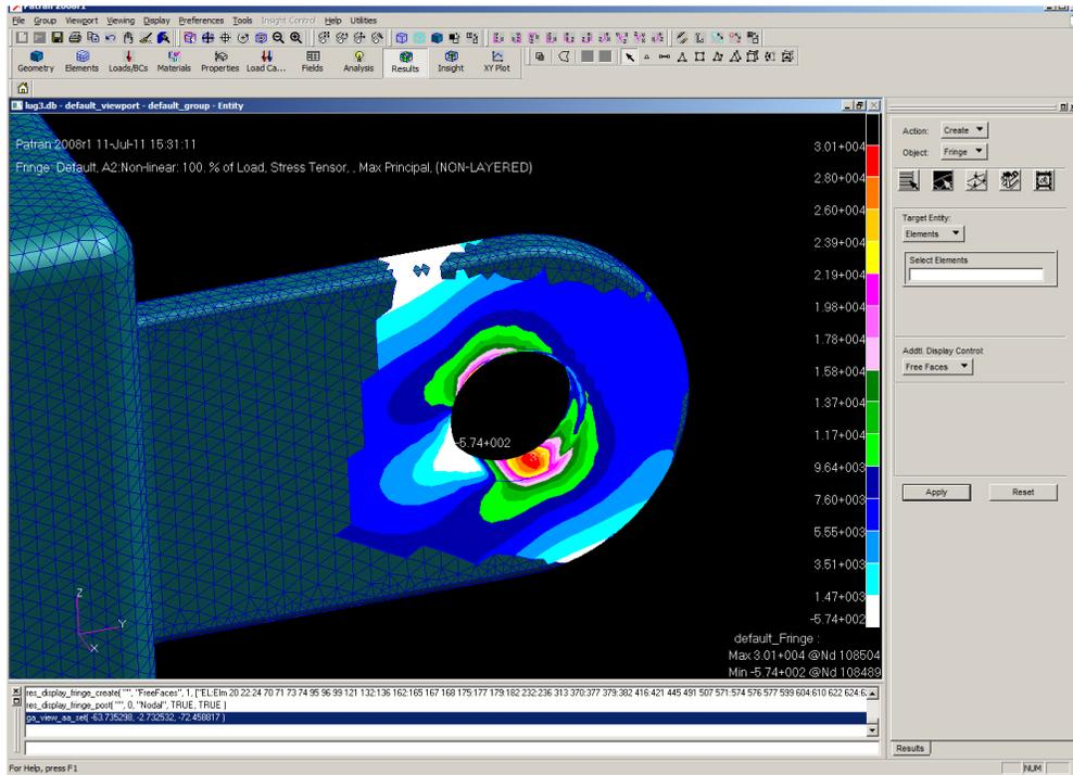
The discrepancy at the radius is explained since as presented earlier the actual load applied by the pressure field was 2,488lbs; thus  $2,500/2,488 \times 46.8 = 47.0$ ksi.
